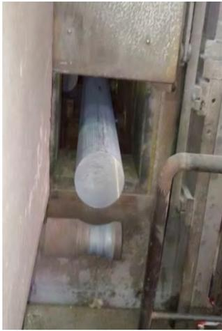
Continuous homogenizing furnace walking beam system
